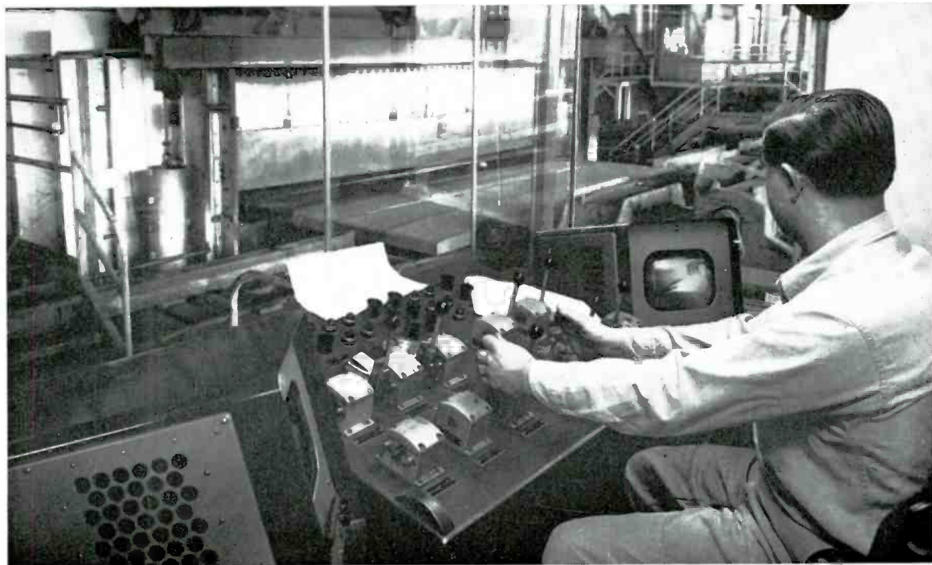
RCA television cameras give furnace operator closeup view of interior of re-heat ovens at Jones & Laughlin steel plant, Aliquippa, Pa.
