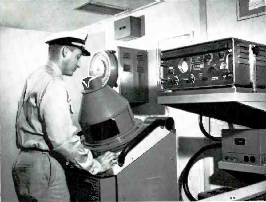
Ocean liner Brasil depends on radar and radio direction finder for safe navigation in the thickest weather.
