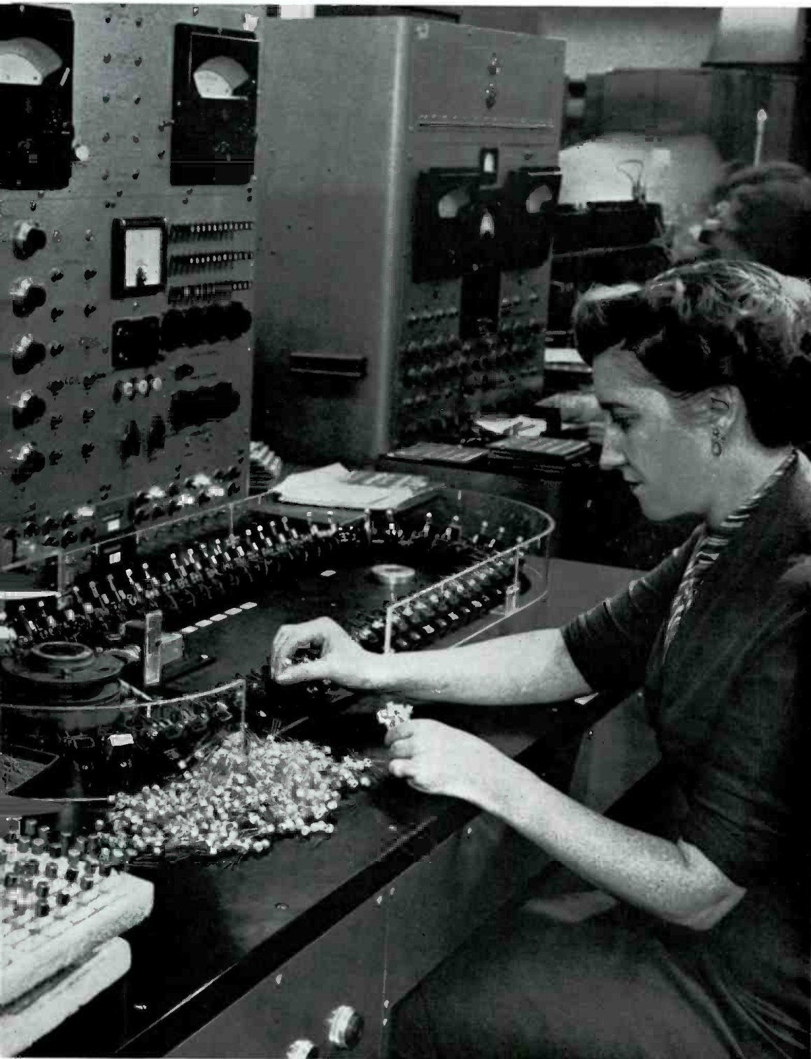
Semiautomatic machine tests 1,600 transistors per hour at RCA plant, Somerville, N. J.
